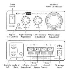
Troubleshooting: No Sound: Verify power is connected, check speaker wires to ensure they are making contact with terminals. Only One Channel of Sound: Check speaker wire connections on the output channel and input connectors found on the amplifier and your speaker that is not producing sound. Popping Noise: Turn down volume prior to powering unit on or off.
